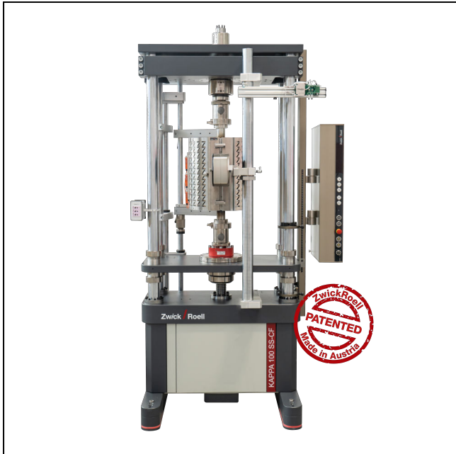
Kappa 100 SS-CF with videoXtens 1-32 HP/TZ and alternatively with contact-type extensometer
